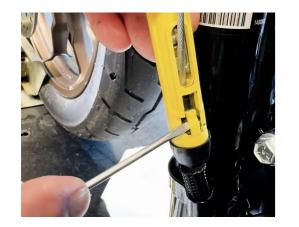
Open the cable adjuster clamp: 8. Use a flathead screwdriver to open the clamp of the adjuster and remove the lower part of the adjuster.
