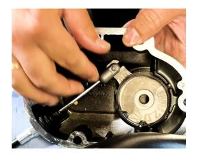
13. Install the new Power Clutch 2.0 segment: Place the new segment into the clutch cover and transfer the three original balls from the old clutch segment.
