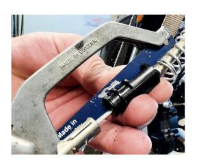
10. Remove the black counter part: Using a small hacksaw, cut off the black counterpart of the cable adjuster and thread out the cable.
