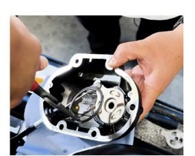
Remove the clutch cover 5. screws: Then, use a snap ring plier to remove the original clutch segment.
