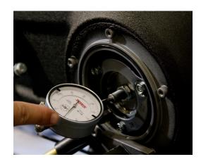
20. Final adjustment check (if you want to be sure): Use a dial gauge to ensure a minimum travel of 1.6 mm at the adjustment screw when pulling the clutch lever. If the travel exceeds 1.6 mm, increase the play at the clutch lever.
