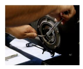
4. Open the clutch inspection cover: Access the primary chain case, loosen the locknut on the adjustment screw, and release the tension.
